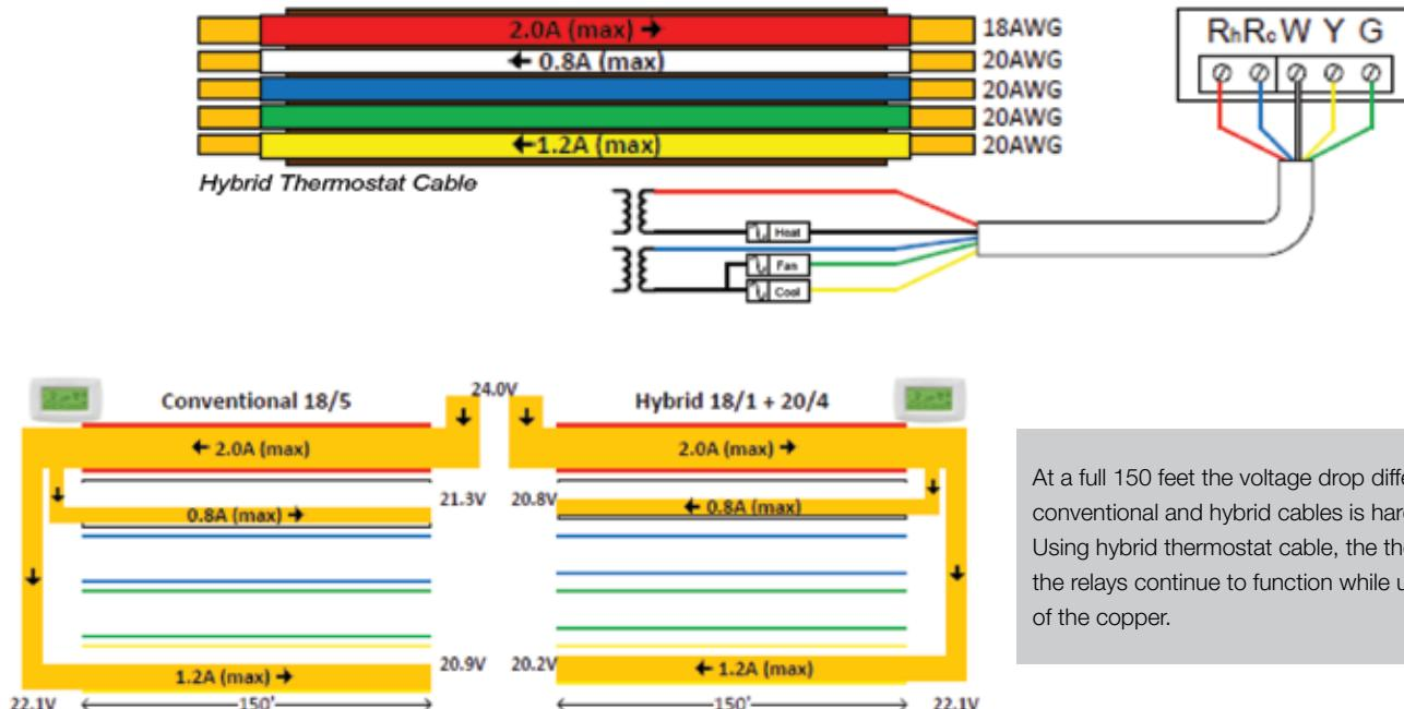
At a full 150 feet the voltage drop difference between conventional and hybrid cables is hardly noticeable. Using hybrid thermostat cable, the thermostat and the relays continue to function while using a fraction of the copper.
