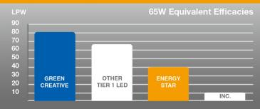
At 81 LPW, this lamp's efficacy is more than 20% higher than the Tier 1 LED BR30 65W replacement industry average and exceeds ENERGY STAR requirements by upwards of 100%. This energy-saving performance makes this lamp a smart retrofit choice for incandescent bulbs.
